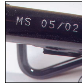
Marking after surface treatment
